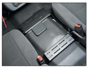
Determine the position of Trak desired and mark location with a pencil on the hump brackets.. Remove the front and rear hump bracket cross support.
